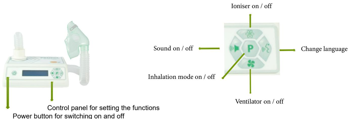
**Display:** The display shows which functions are switched on or off.
